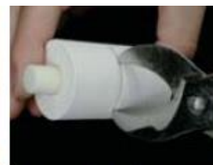
Final removal with a plaster nipper
