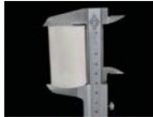
Carefully level the ring so that the top and bottom are perpendicular to the sides of the ring.
